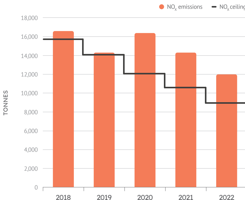
Figure 8: Nitrogen oxide emissions from Bosnia and Herzegovina's NERP coal plants, compared to the allowed emissions ceilings, 2018 to 2022
